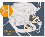
Clamp the red and blue line on the clamp symbol. Apply a third clamp downstream of the flow/bubble sensor.
