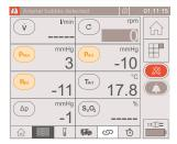
With the tubing free of liquid, zero three pressure sensors ( $P_{\text{Ven}}$ ,  $P_{\text{Art}}$ , and  $P_{\text{Int}}$ ).
