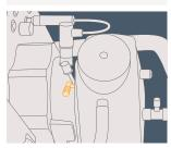
Close the de-airing membrane with the yellow protective cap.
