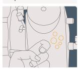
Tap the tube system and the HLS Module with your hand to remove any gas bubbles.
