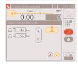
Calibrate the flow/bubble sensor.
