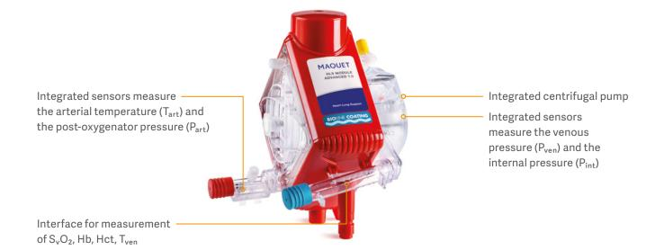
The HLS Set Advanced includes a high performance oxygenator with integrated centrifugal pump, pressure and temperature sensors (HLS Module Advanced). Integrated non-invasive sensors help to increase the safety during the application and avoid the need for external measuring lines.
