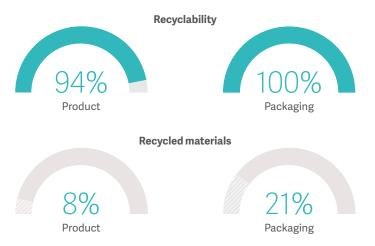
The following materials are considered recyclable: Steel, Alu, Bronze, Brass, Copper (except cables), Cardboard, Paper, Thermoplastics (PMMA, PVC, ABS, PC, PS, PET, PE, PA, PP, POM). Thermosetting plastics, elastomers and other materials not listed are considered non recyclable. Recycled content evaluated in the study but requires documented trail in the value chain.
