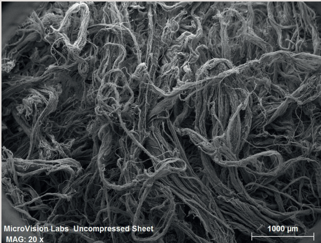
Getinge OEM collagen – microscopic view of fibers
