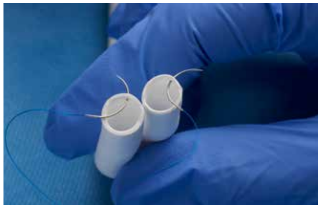
Wall thickness of standard wall vs. graduated wall
