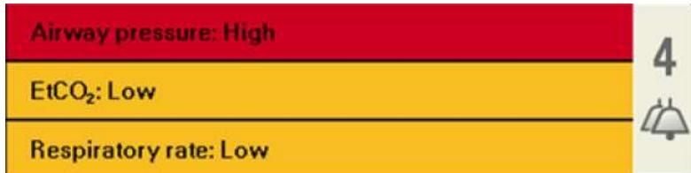
The alarm area on the screen can display up to three alarms, listed in order of severity. Should there be more ongoing alarms, a number will be visible to the right (in this case 4). Pressing the number shows up to 10 ongoing alarms. For previous alarms press “trends” on the same page.
