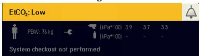
An anesthesia machine is designed for the presence of a trained specialist to be by its side. **There are neither lamps nor remote monitoring. Once an alarm is no longer valid, it is not audible or visible anymore and the sound of the alarms in general are lower than an ICU-ventilator.**
