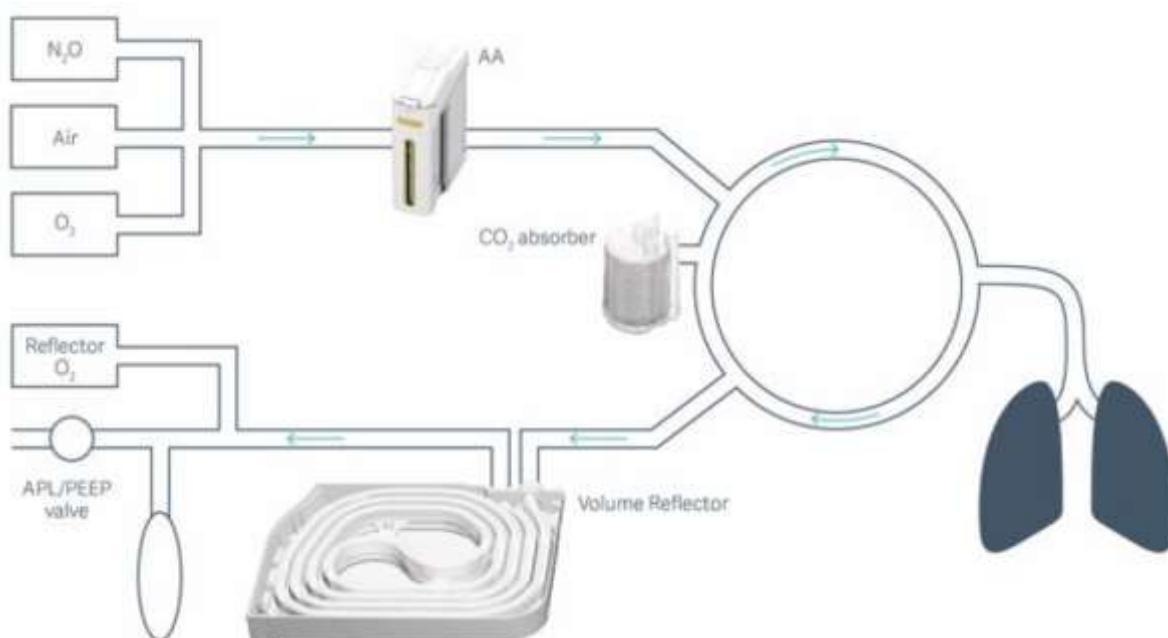
If non-rebreathing is desired, we recommend the user set the fresh gas flow higher than the patient's expired minute volume. If the user sets the fresh gas flow to 20 l/min, the system is designed to automatically adjust the fresh gas flow to just above the patient's minute volume and, thus, guarantee a non-rebreathing system.
