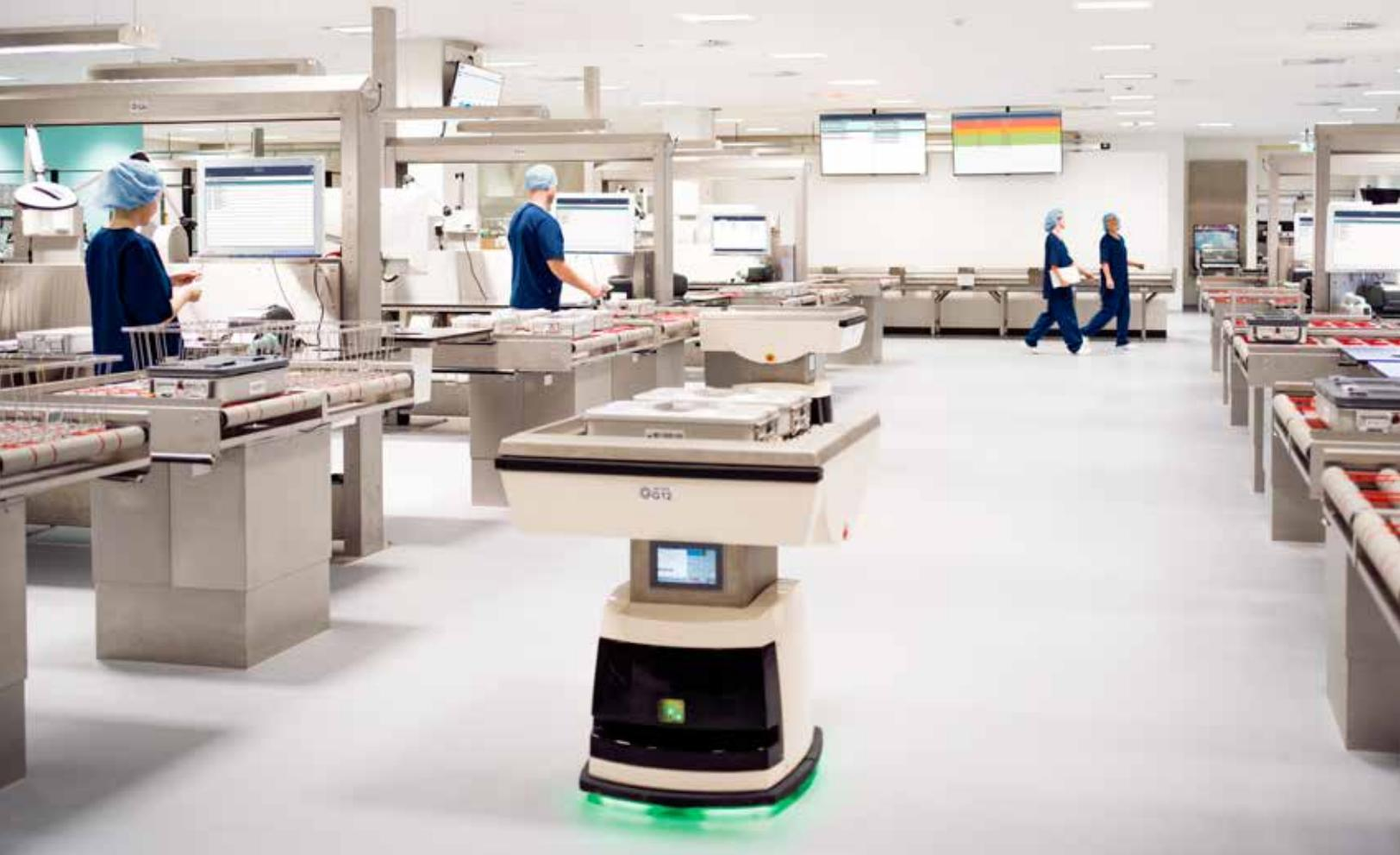
T-DOC driven AGV (Automated Guided Vehicle) transports instruments to and from washing and packing tables.
