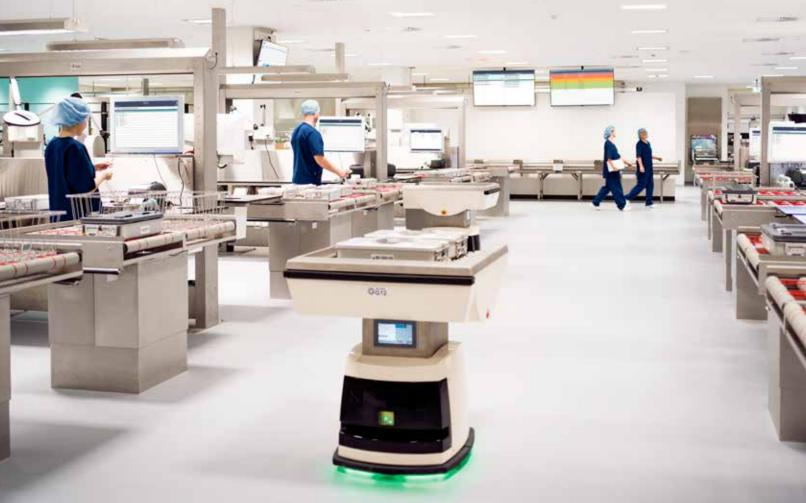
T-DOC driven AGV (Automated Guided Vehicle) transports instruments to and from washing and packing tables.
