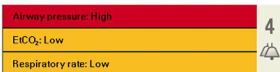
The alarm area on the screen can display up to three alarms, listed in order of severity. Should there be more alarms that are ongoing a number will be visible to the right (in this case 4). Pressing the number shows up to 10 ongoing alarms. For previous alarms press “trends” on the same page.
