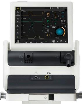
Servo Compass® clearly visualizes when driving pressure or tidal volume per kilogram of predicted bodyweight are off target.¹
