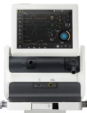
Servo Compass® clearly visualizes when driving pressure or tidal volume per kilogram of predicted bodyweight are off target.
