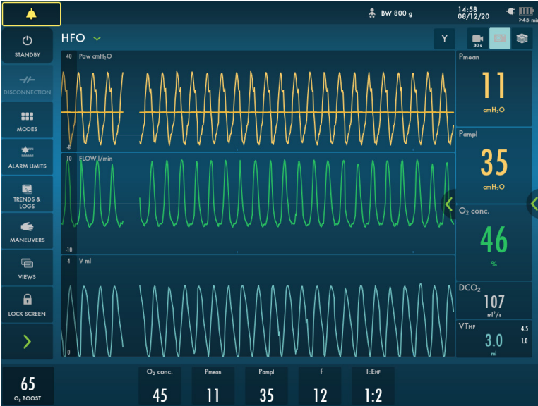
High Frequency Oscillation (HFO) mode, pressure amplitude control.
