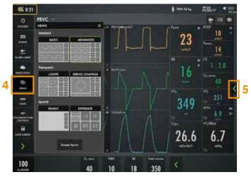
53. If SERVO COMPASS view is available, tap on the **SERVO COMPASS**.
