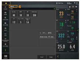
36. Change the **TRIGGER** value to pressure triggering -1 cm H<sub>2</sub>0.
