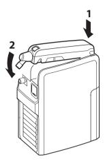
Hinge the expiratory cassette and press it firmly down into lock position.
