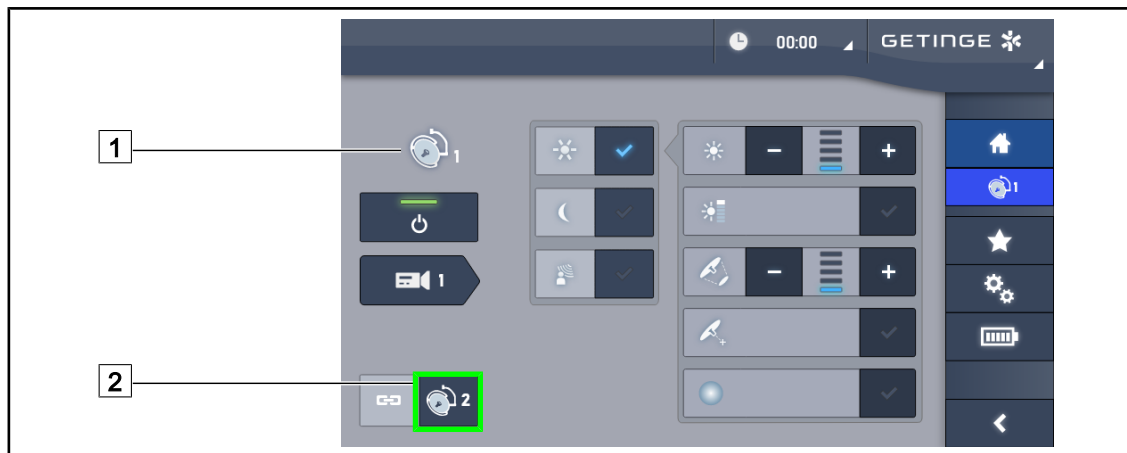
Fig. 60: Synchronising the lighthead
