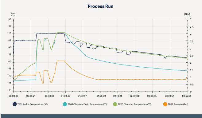
The process trend illustrates a typical process using default parameters. The pretreatment phase is naturally convected dry heat and the post sterilization phase is natural cooling.
