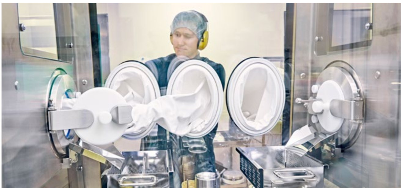
DPTE® component transfer at Octapharma SVP-filling line in Stockholm
