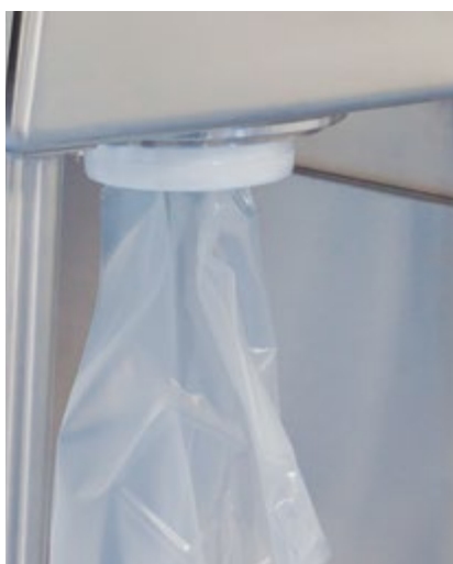
Removal of solids & liquids Samples to QA/Waste via DPTE®
