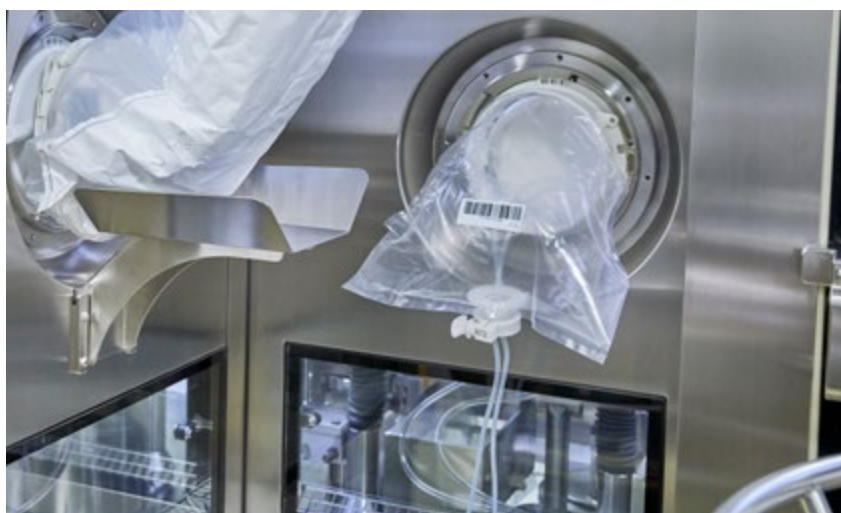
Liquid Transfer DPTE® single-use technology
