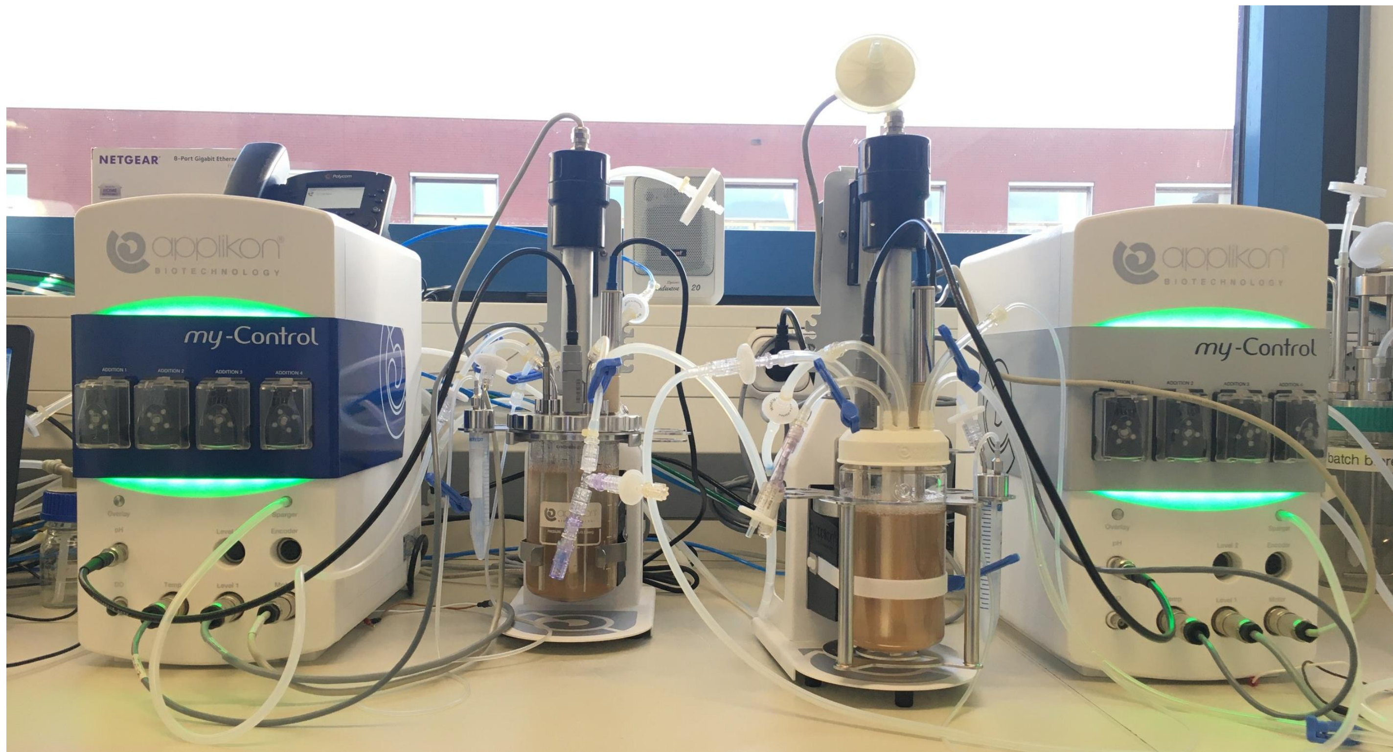
Figure 2: Experimental reactor setup with miniBio (left) and Appliflex ST (right) bioreactors.
