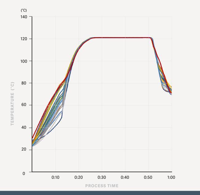
Thermal mapping of 24 thermocouples (TC) placed inside a typical 2mL prefilled syringe nest during validated sterilization cycle in a 9 cubic metre chamber.
